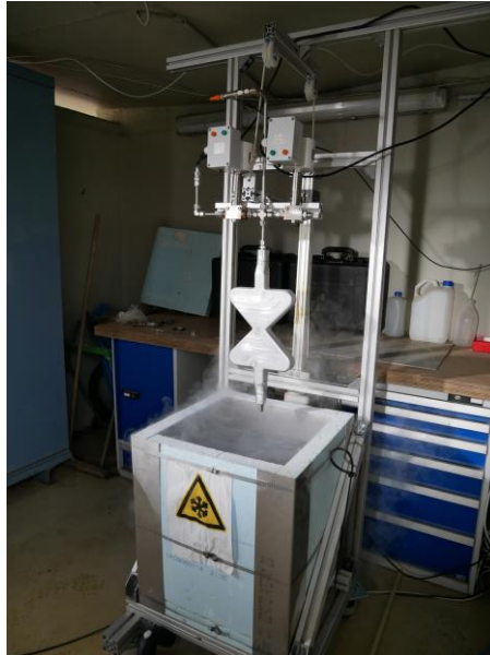
Figure 1. Moderator vessel (BF1, Generation 2 moderator for the ESS) prepared for burst test mounted on a linear actuator with installed pressure sensor and cryogenic high pressure magnetic valves and a liquid nitrogen bath below
